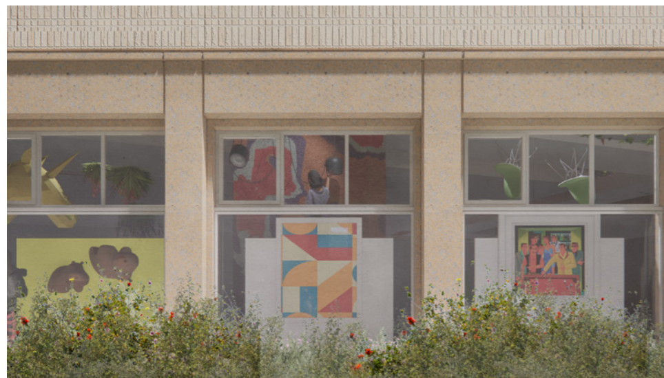
Typical studio facade treatment. The low wall create a display window for the artists which maintaining privacy and passive surveillance.
