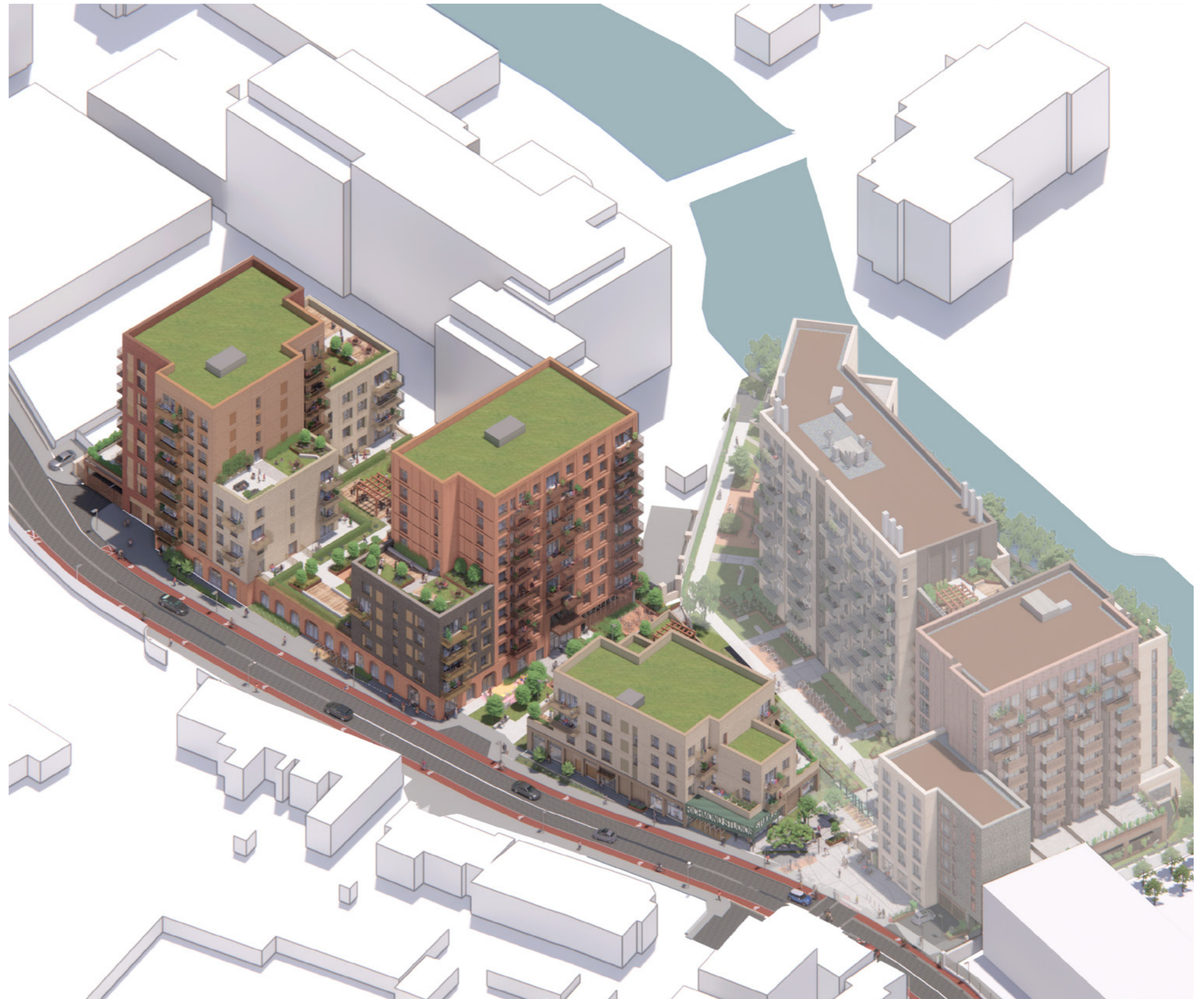
The buildings vary in height, bulk and form to provide visual interest and to break up the massing
