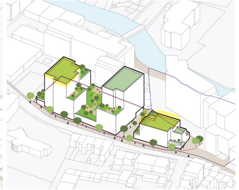
Current Site Massing, one storey removed from Block A, and one storey added to Block C - Block A = 4-Storeys, Block B = 10-storeys and Block C = 9-Storeys
