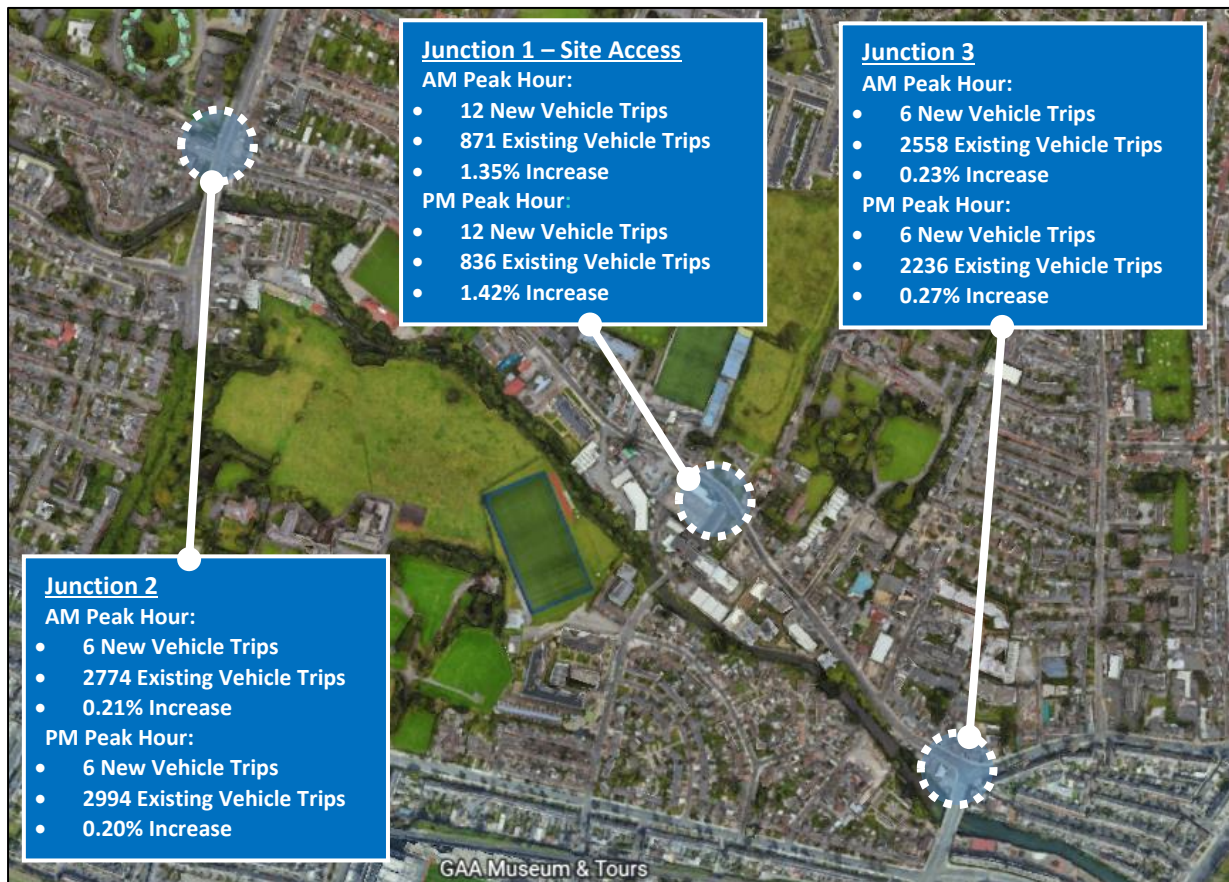
Figure 5.3: Increase in Vehicle Trips Generated at Site Access and Key Off Site Junctions (2040 Do-Something)
